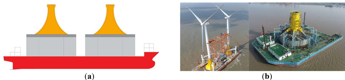
Figure 9. Bucket foundation-tower-unit integrated floating transportation and installation technology. (a) Traditional dry tow floating transportation; (b) New ship-under air-floating op towing technology.
