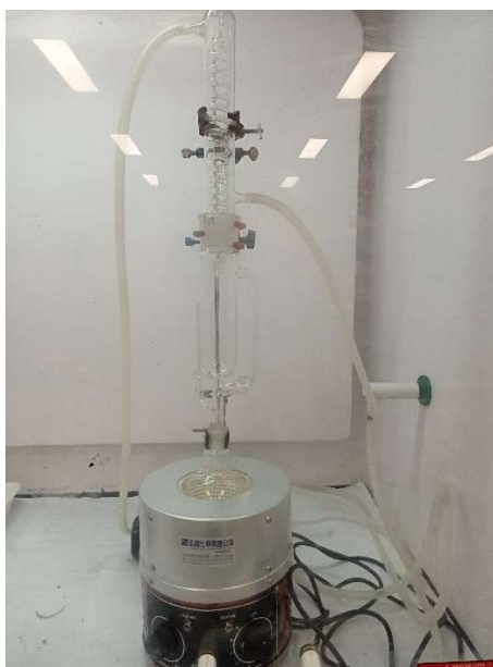
Figure S2. Reflux setup for the purification of SWCNTs.
