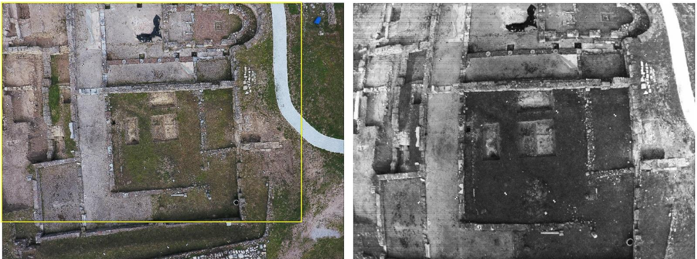
Figure 6. Two images with flight directions from south to north. On the left, the RGB image of the RGB Phantom. In the yellow frame the surface covered by the images (RGB or MS) of Sequoia+. On the right, the Green band of the MS image of Sequoia+.
