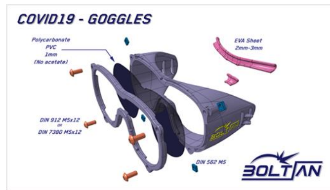
Figure 5. Components of 3D printed goggle frame for protective eyewear [71].
