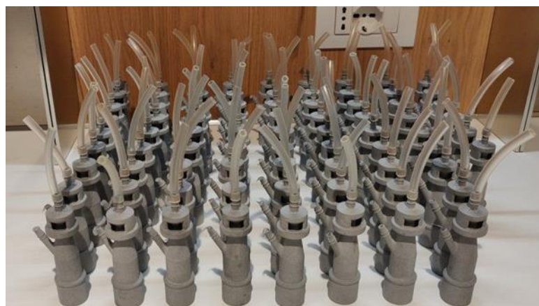
Figure 6. An Italian engineering startup created a 3D-printed venturi valve to help patients with difficulty breathing. (Image taken from: https://www.bbc.com/news/technology-51911070 ).
