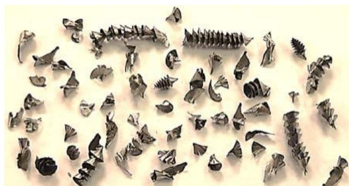
Figure 5. Chip morphology after UVAM [46].
