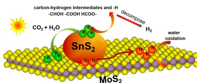
Figure 9. Schematic illustration of H 2 generation process in CO 2 saturated solution on SnS 2 /MoS 2 catalyst.
