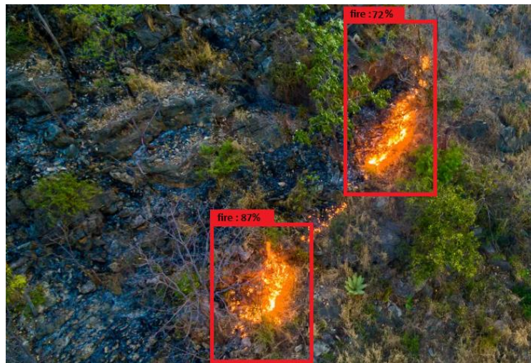
Figure 4. Fire detection using RGB camera and AI methods.
