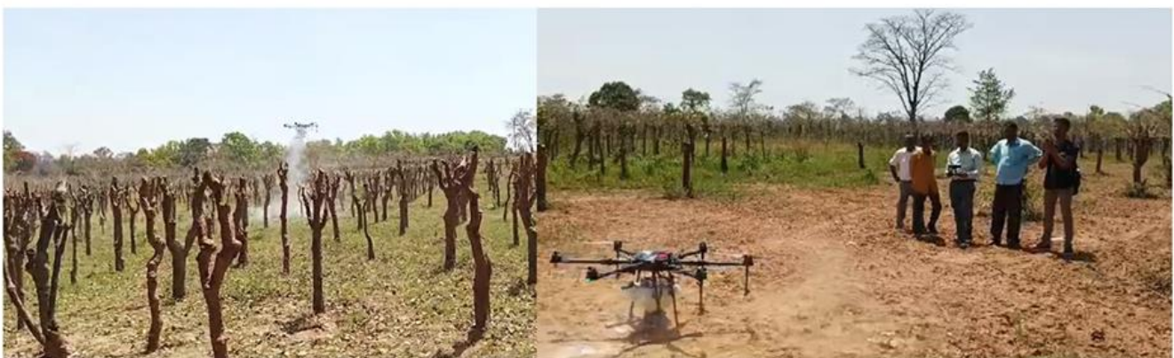
Figure 3. Lime and bleaching powder spraying using a hexacopter drone in Arjun and Asan field demonstrated at CSB-CTRTI, Ranchi, India.
