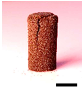
Figure 11. Fractured cylindrical part after compressive test (scale bar: 5 mm).
