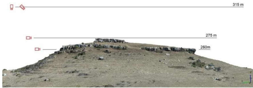
Figure 3. The various flight heights for vertical, inclined and horizontal image collection (perspective from the west).
