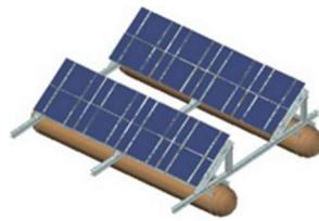
Figure 13. The FPV floating structure in Korea.
