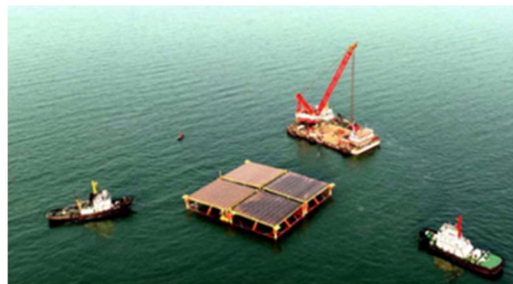
Figure 18. The first semi-submersible offshore FPV platform in China.
