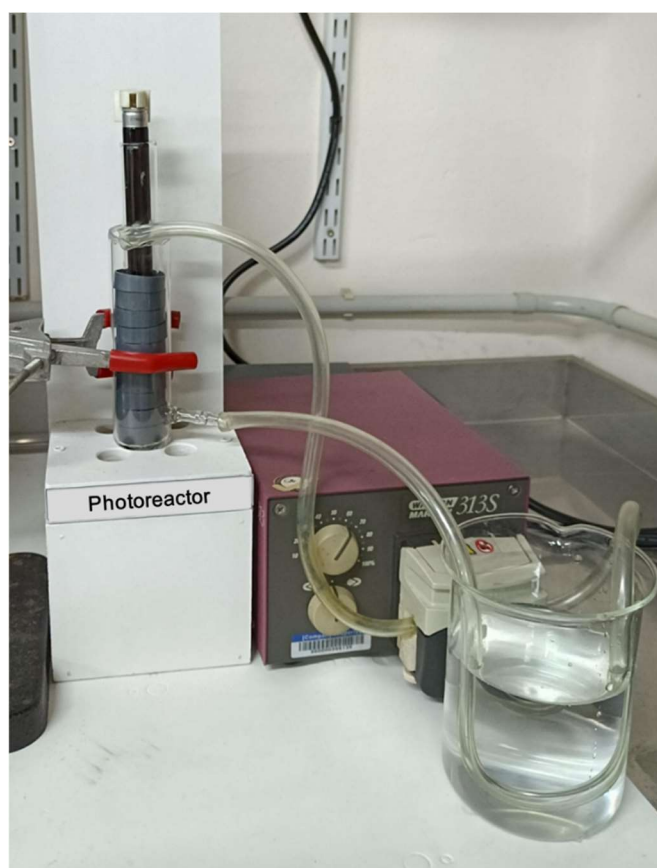
Figure 8. Photograph of the photocatalytic irradiation setup.
