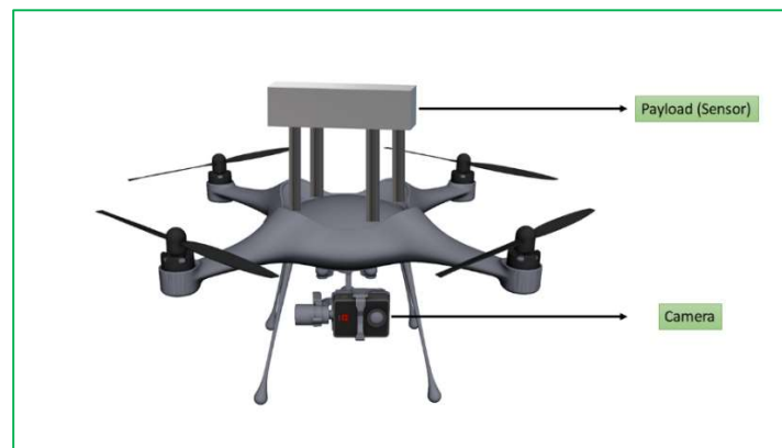
Figure 6. Fixed location for mounting of environmental Sensors.
