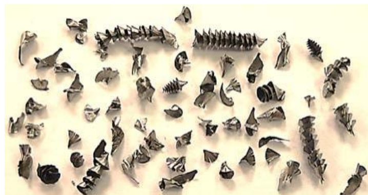
Figure 5. Chip morphology after UVAM [46].
