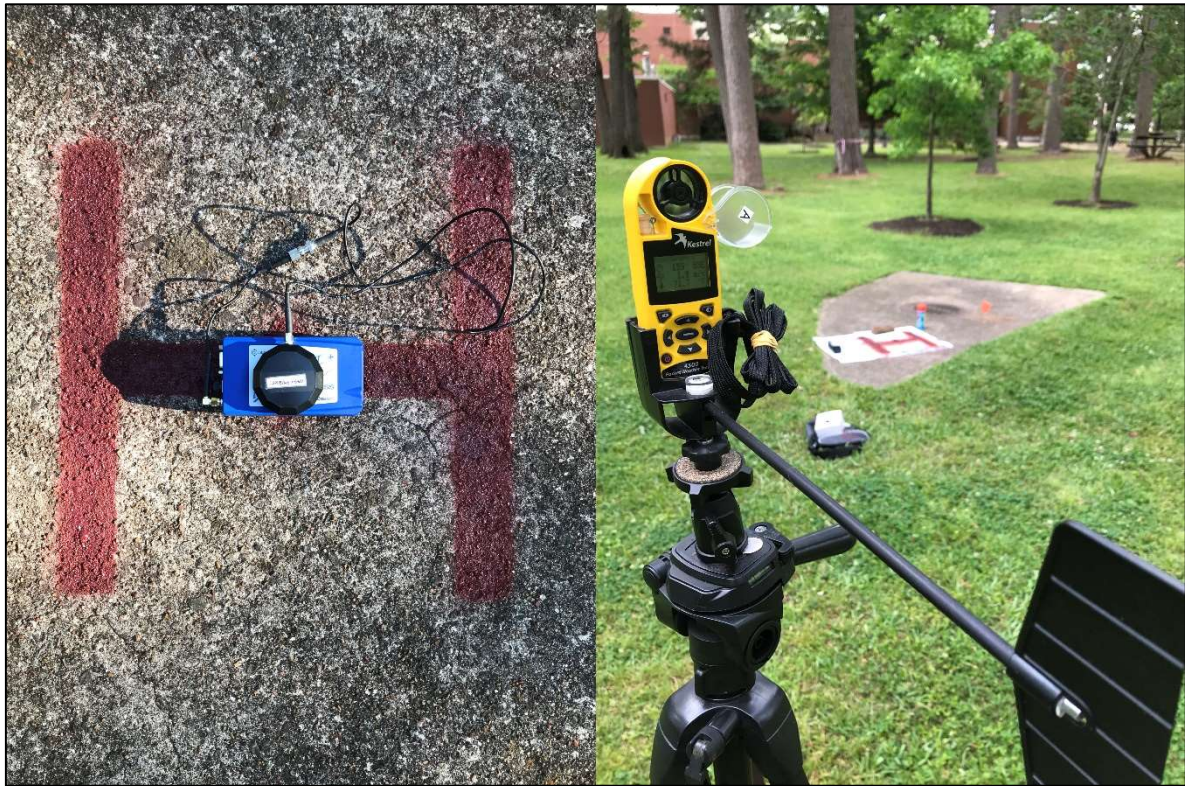
Figure 1. The painted launch pad with a submeter GNSS receiver recording its geographic coordinates (left) and the launch pad with a weather meter in the foreground (right).
