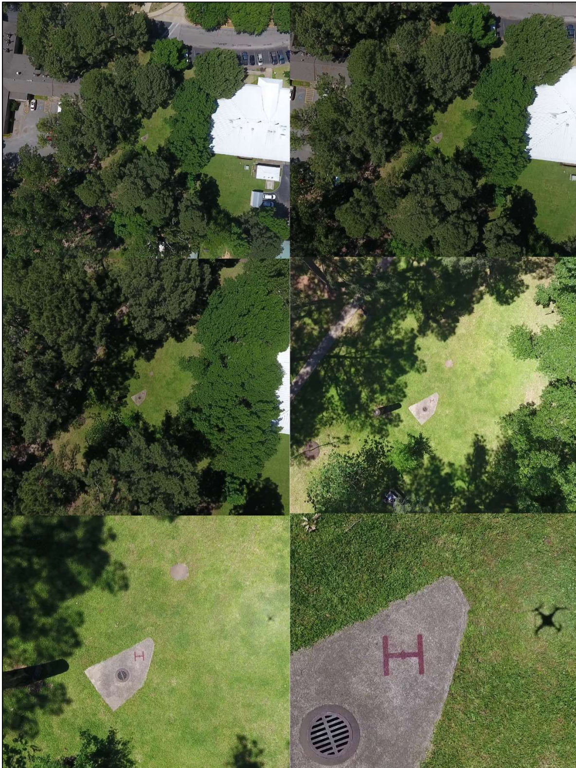
Figure 2. A sequence of downward views from a drone during the return-to-home descend process.
