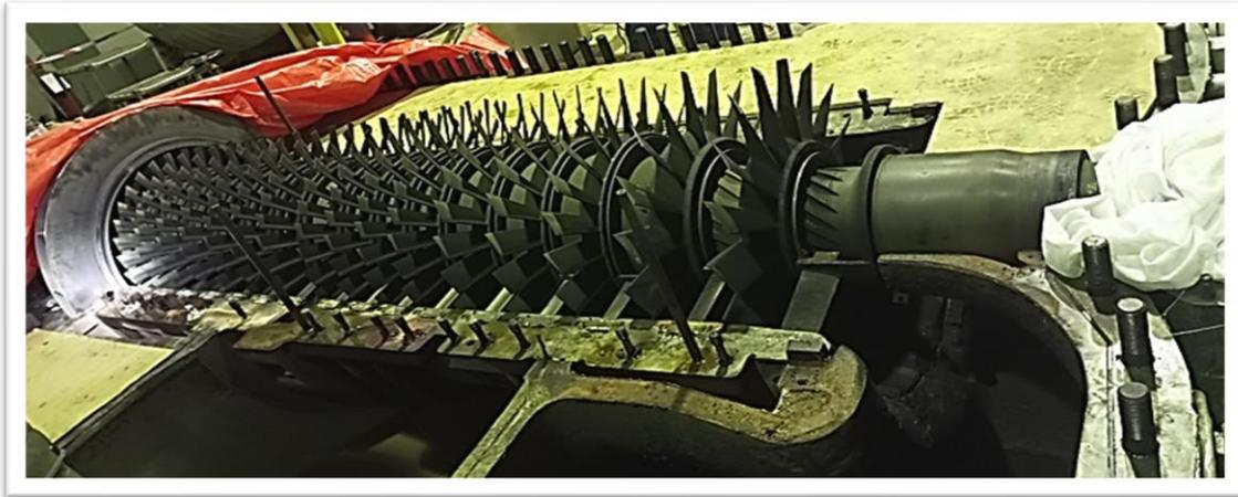
**Figure 5.** Compressor and rotor casing.
